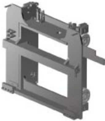
Carriage for attachment with leveling in twistlocks, standard on DCF70-90 for single stacking
