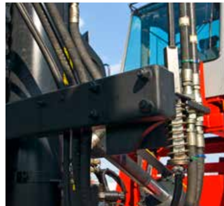
Fewer components makes for increased reliability, only two hoses and one harness runs over the mast wheel.
